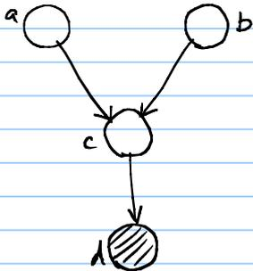
$$\begin{aligned} p(a, b \mid d) &= \frac{p(a, b, d)}{p(d)} \\ &= \frac{p(d|a, b) p(a, b)}{p(d)} \\ &= \frac{p(d|a, b) p(a) p(b)}{p(d)} \leftarrow \textcircled{1} \text{ F!} \end{aligned}$$
